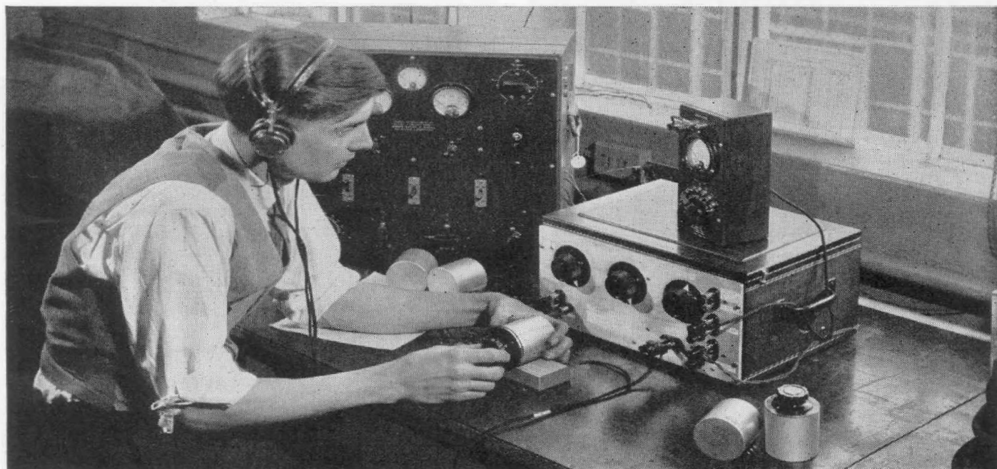
FIGURE 5. Inspecting TYPE 653 Volume Controls for noise. Every General Radio volume control is individually tested for noise, attenuation, and impedance, as well as the usual mechanical inspection
